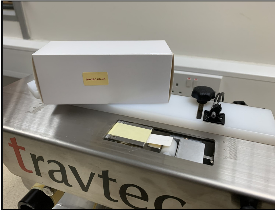
Labels semi-automatically applied to cartons on the Tiny Labelino
